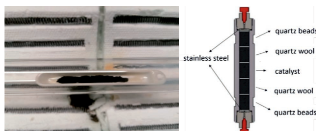
Figure 2. a) The prepared catalyst, b) Schematic view of the applied catalyst column.
